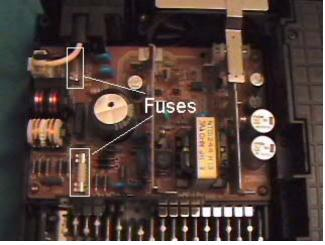
Remove the 4 screws as indicated in the diagram and lift the power supply board out and check the fuses. The power switch and other checks are the same as on the other board.
