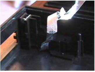
Use a small bladed screwdriver to lift up on the back of the assembly and it will come loose. Be careful when pulling the buttons through the holes in the console so that they do not get hung up and break.
