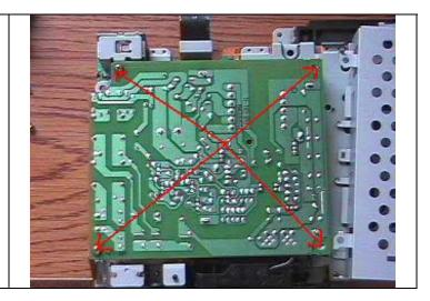
Every version of PS2 has a slightly different set of fuses in it. To convert the numbers on the fuses to an actual value take the number and multiply by .04. For example, if the number on your fuse is 25 CCP2E25 then you take 25 \* .04 = 1.0 or 1 amp. You would use a 1 amp fuse to replace this one. If you end up with a weird amperage like .52 just use a .5 amp fuse. You just need something close as possible to the actual value to keep things working safely.
