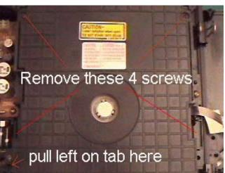
Plug the unit in and hit the eject button so the tray comes out and then unplug the unit. Lease the tray in the out position. You then need to remove the screws that are holding the rods that the laser assembly travels on. (*see picture*)
