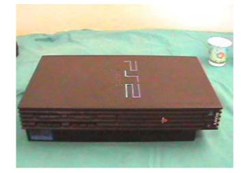
Pull up on the cover from the back and work it free and lift about 1/2 inch. Move the shell forward a little, sideways, so that the **Eject/Reset buttons** are **not blocking** the shell and the CD tray comes clear, and it can be lifted off. Just play around with it a little and you should get it.
