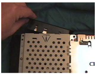
H. Now that the shields are removed you are going to lift and fold back the expansion slot to reveal the laser voltage adjustments. **BE VERY CAREFUL-YOU WILL BE MOVING RIBBON CABLE AND CAN BREAK IT IF NOT DONE CAREFULLY.**
