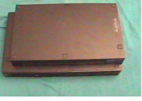
E. The PS2 shell should now be ready to remove. ONLY the UPPER side (with the PS2 logo) needs to be removed for this step - Leave the BOTTOM side on. **WARNING-Be** very careful when taking the upper shell off, or you could damage the PS2.
