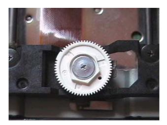
5. Turn the wheel about 1/8 of a turn. Put the CD tray cover back on. You DO NOT need to put the screws in. just hold it down lightly with your hand. Put in one of your game discs and push it in and see if it works. You may have to use the browser to load each disc you are testing.
