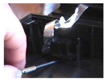
Once the assembly is loose you will be able to remove the cable (or reattach it). As you can see the blue side of the cable is facing towards the circuit board.
