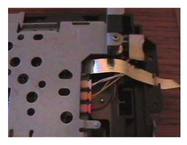
Carefully reassemble the console. You may want to check the operation of the cable before putting the top cover back on. Just remember to be careful when working on live equipment.
