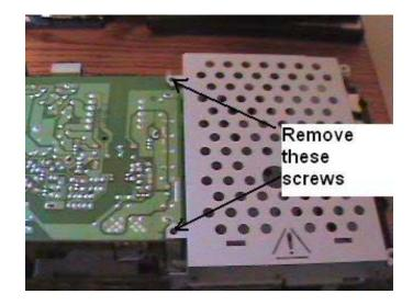
Once the cover is removed you will be able to see where the ribbon cable connects. The blue side is facing up in this picture.
